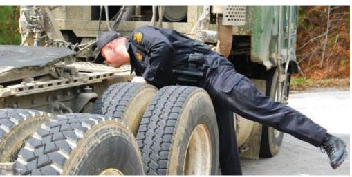
The largest percentage of all outof-service violations occurs from brake-related violations during roadside inspections. Trucks with improperly installed or poorly maintained brake systems can pose a serious risk to the driver and public safety by reducing the braking capability and increasing stopping distances of trucks and buses, according the CVSA.
